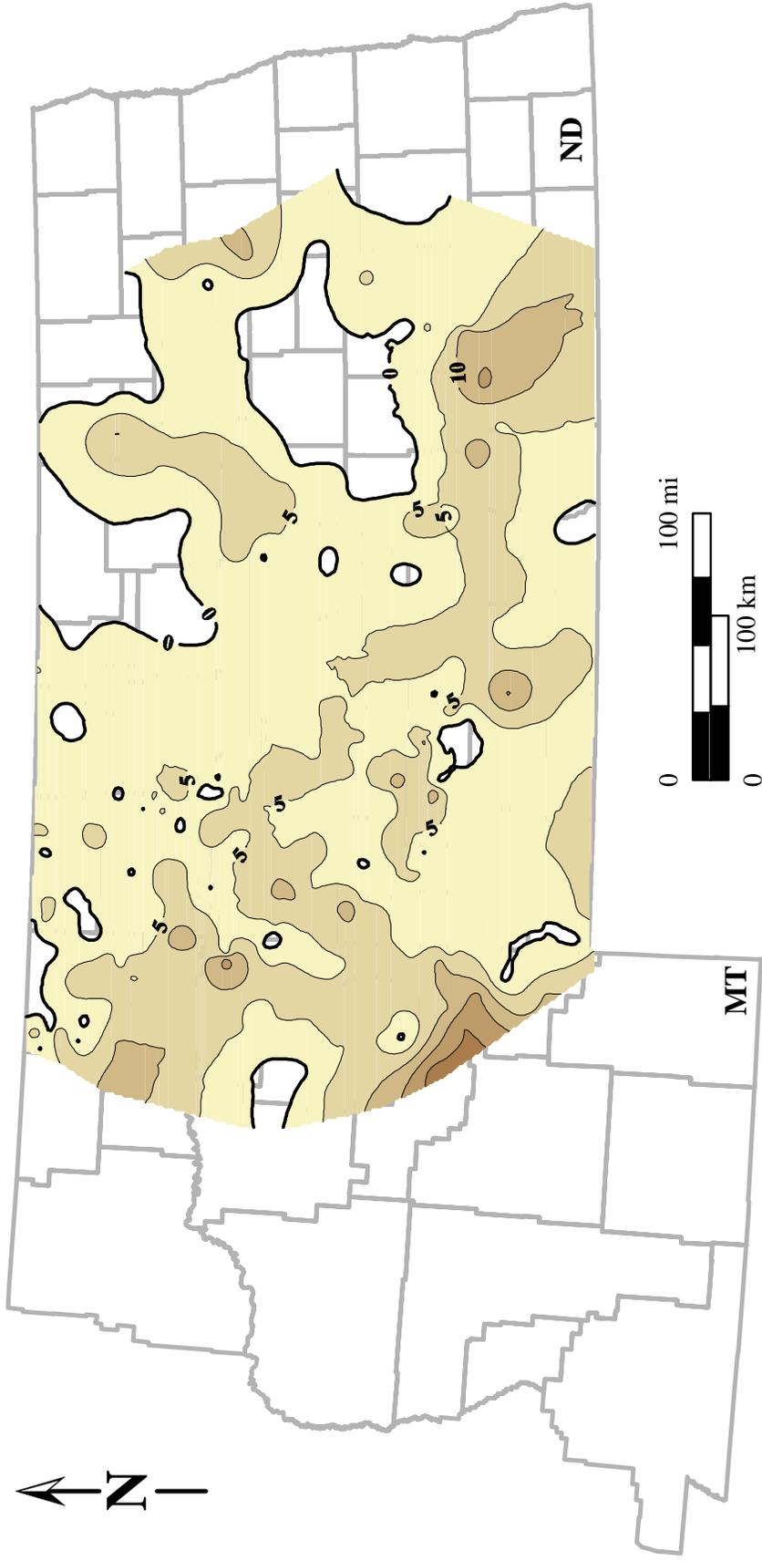
**Figure 6.** Distribution and thickness of sandy unit S1.
