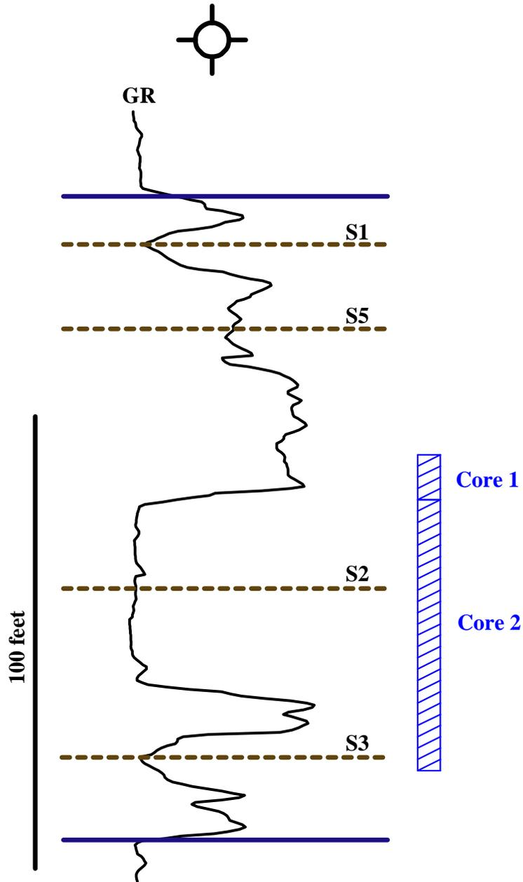
**Figure 36.** Gamma-ray curve and cored interval for the Amerada-Hess #36-44 Federal well Sheridan County, Montana.
