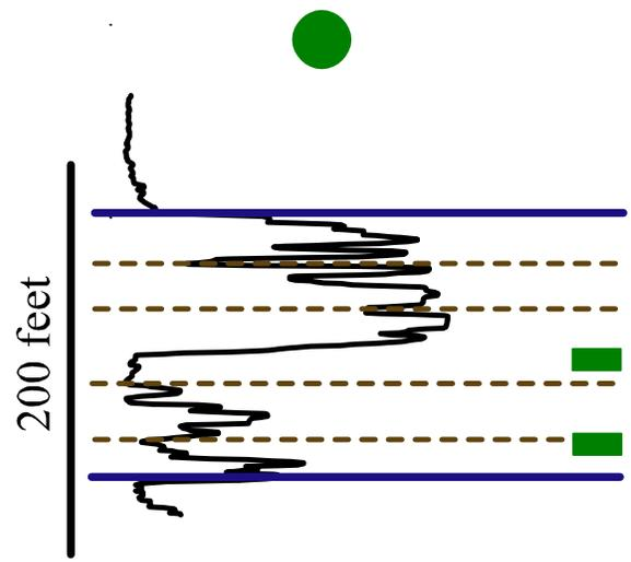
**Figure 35.** Locations and gamma-ray curves for the Sun Tronson and the Enserch Aasheim-Clark wells, Sheridan County, Montana. Dashed lines represent the centers of the sand bodies. Heavy bars are the tested intervals.
