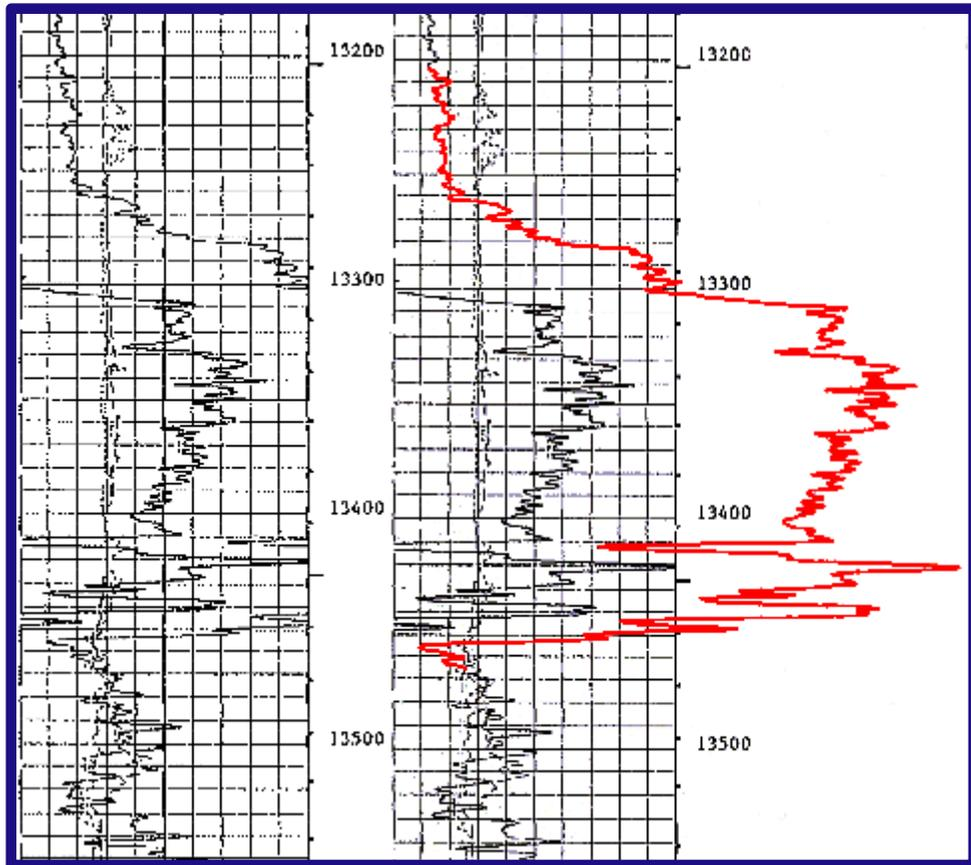
**Figure 4.** Example of elimination of “off-scale effect” and digital conversion of trace. Left - original gamma-ray log trace; right - gamma-ray log trace overlain by spliced trace.
